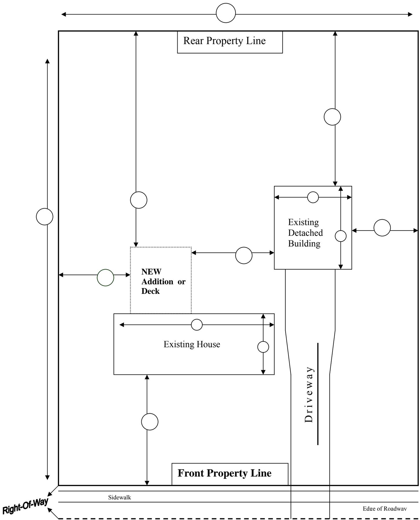
This site plan is for example purposes only. A plan including location, dimensions and setback from property lines for all existing and proposed structure is required for review. Although a scale is not required, all dimensions must be true to the parcel and reflect setback from actual property lines, rather than sidewalk, curb or roadway.
